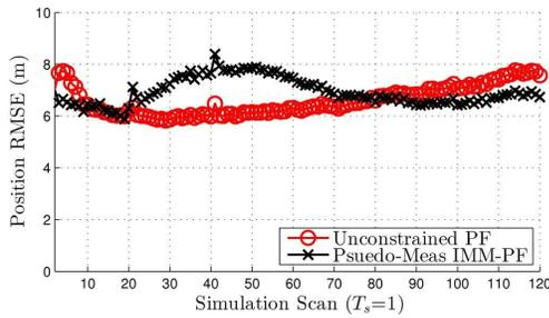
Fig. 7. Position RMSE over time for the standard *Unconstrained PF* and the *Pseudo-Measurements IMM-PF*. The filter does not overcome the increase in error due to the constraint violation for  $k \in [21, 40]$ .
